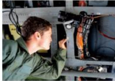
Instrumenting an HH-60G 308 Beam
